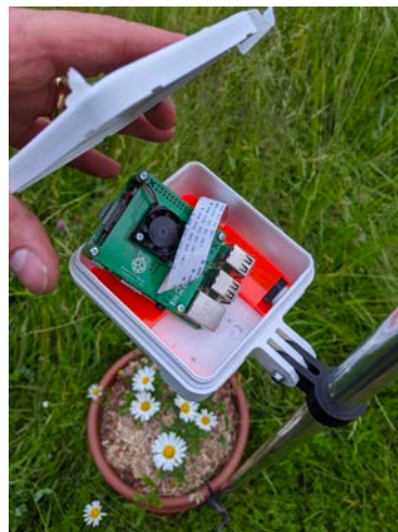
Plugging in PoE requires opening this (bad) design
