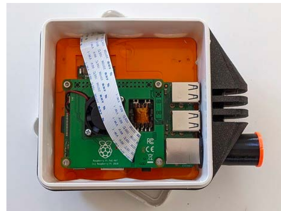
Enclosure (w/ PoE shield, adapter, plug)
