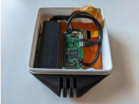
Hardware (w/ Pi Zero, Pi Cam v2, PoE)
