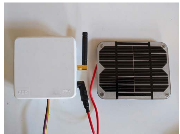
Enclosure (w/ 1W solar panel)
