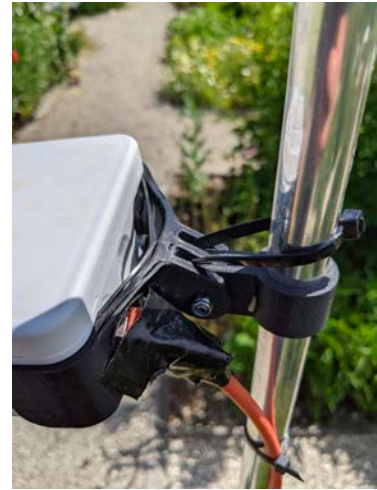
Sun damage due to PLA instead of UV-proof ASA
