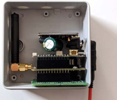
Modular electronics (w/ LoRaWAN)
